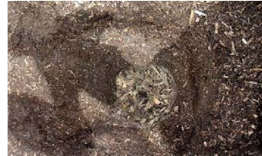
Figure 1. Partly dried out biofilter. Courtesy of REINLUFT Umwelttechnik, Germany.
