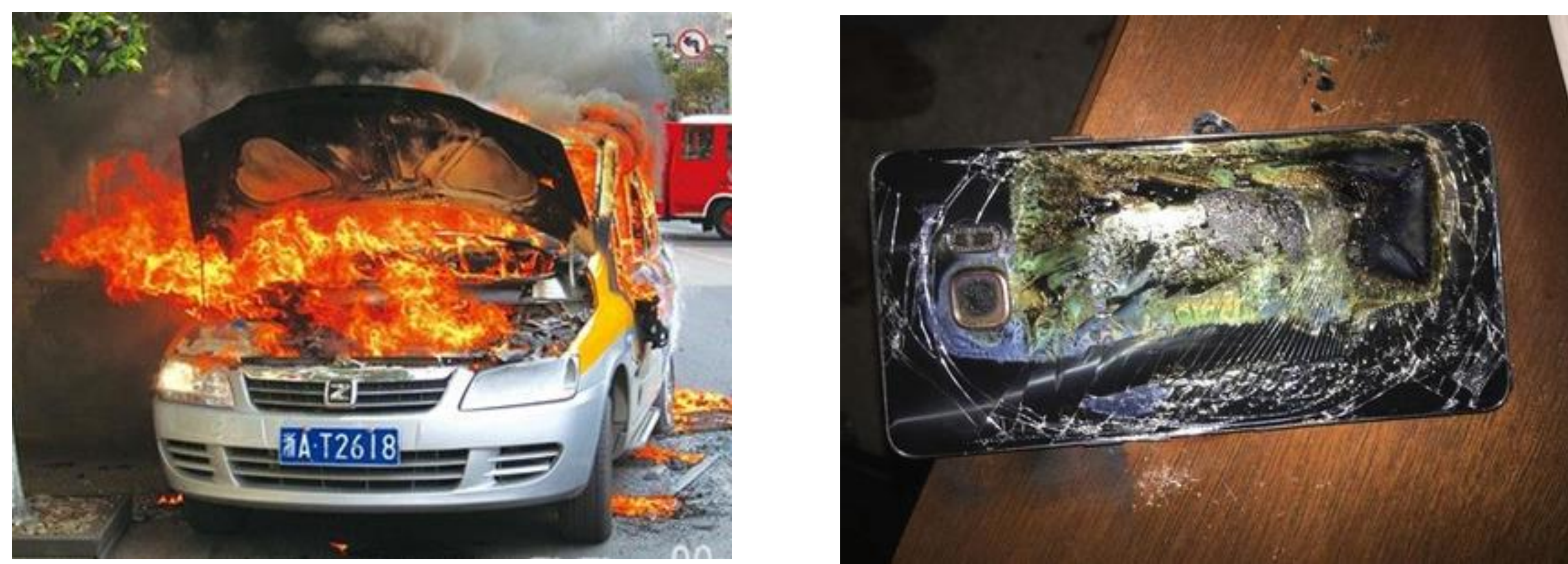
Figure 1. Thermal runaway caused fire of lithium ion batteries.
