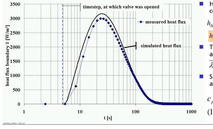
Heat transfer coefficients  $h_{HF} = 400 \text{ W/m}^2 \text{K}$  $h_{Ad,m} = 500 \text{ W/m}^2 \text{K}$ Thermal conductivity adsorbent  $\overline{\lambda}_{Ad} = 0.2 \text{ W/mK}$
