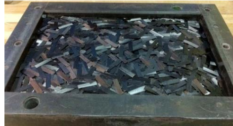
Figure 1. Randomly oriented strands ready to be processed in a flat plate.
